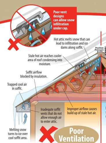
High airflow vents such as the PROVentilator allow faster air movement through the attic. Attic air that does not move can cause home damage such as moisture and mold.
