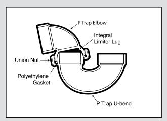
An integral limiter lug prevents the P Trap Elbow from pitching backwards providing the correct outlet slope for drainage. The polyethylene gasket ensures a leak proof connection in almost any installation situation.
