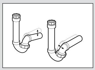
The ball joint union connection allows the P Trap Elbow to swivel up to 10° from vertical, in any direction, except directly backwards.
