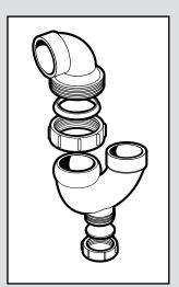
No need to tighten the union nut by mechanical means causing damage and possible leaks. The oversize union nut can be simply hand tightened for a positive seal.
