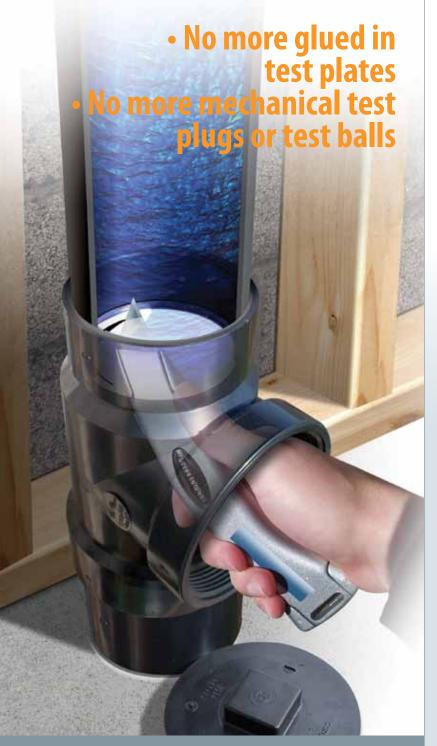
By puncturing the PVC membrane with a utility knife, wastewater is drained slowly, avoiding the typical torrent of wastewater mess with other test methods.
