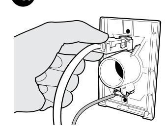
After drywall is complete, plug the E-box into the back of the new ElectraValve® and attach the low volt wires.
