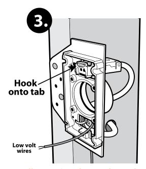
Install mounting plate to the stud. Hook the E-box plug to the mounting plate tab and wait for drywall completion.
